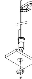
the mounting nut can be locked by fixing the two inserted screws
